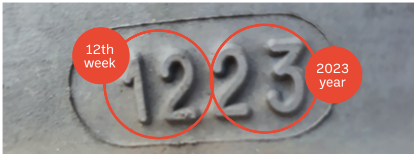
Figure 7: Production Date Code 1223 = 12th week of 2023
